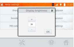
Use "+" and "-" buttons to set the desired brightness and confirm it by pressing **OK**.
