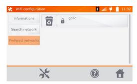
After clicking **Prefered net-works** button, the meter will display networks saved in its memory.
