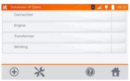
The meter has 4 default types saved in its memory. Use  $\bigoplus$  button to add a new type of the tested object.
