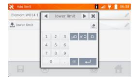
Enter the lower limit. Use button to go to the upper limit setting. You can set only one of the limits.
