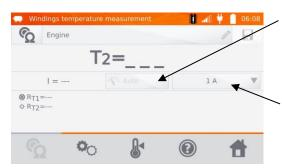
The method of supplying the measuring current is non-adjustable and set on Auto mode - the measuring current is limited to a value not exceeding the set value.
