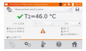
R<sub>T1</sub> – resistance of the cold winding
