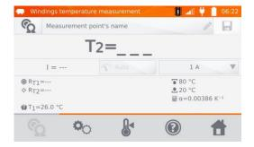
8 Connect the meter to the motor windings. Press START/STOP.
