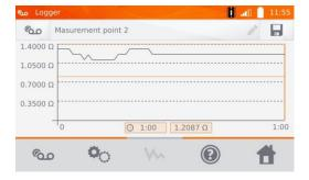
Use W button to display the graph of resistance over time - both during the logging process and after its completion.
