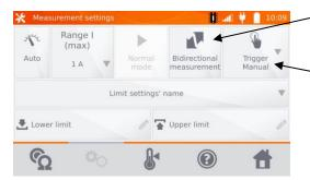
Switching Unidirectional/Bidirectional measurement.
