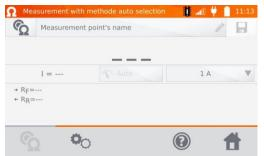
The measurement is performed as in the case of testing the inductive objects If based on the difference between the instantaneous and average resistance during the result stabilization, the meter determines that the object is resistive, it will complete the measurement faster.
