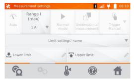
If necessary, select temperature limits from the database (click **Limit settings' name**) or set the required limits for the performed measurement by clicking **Lower limit** and/or **Upper limit**.
