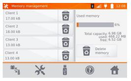
This option allows you to read the % of the used memory and to clear it: after pressing **Delete memory** all clients are deleted with their objects and measurement results. Use button located at the client to delete individual client.
