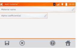
Enter and save the material and  $\alpha$  coefficient, using the same method as described in section 2.3.4.
